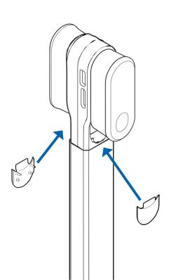
Lock the lock so that the two cover plates are locked.
