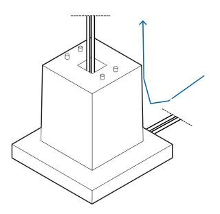
Feed the electrical supply lines and, where applicable, the Ethernet cables through the concrete foundation. At the top, at least two metres of each supply line should still be available to you.
