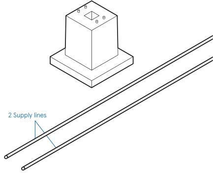
Lead the two electrical supply lines to the installation site. There, keep at least 2,000 mm cable length available at the installation point in order to be able to later feed the feeds through the ePOLE duo and be able to connect the eCLICKs.
