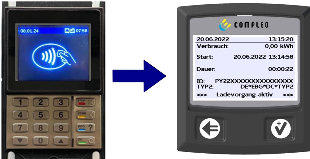
1. End the charging process by presenting the same RFID card or optionally on the vehicle.
