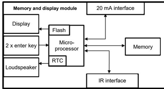
The adjacent image shows the internal relevant components of the SAM.
