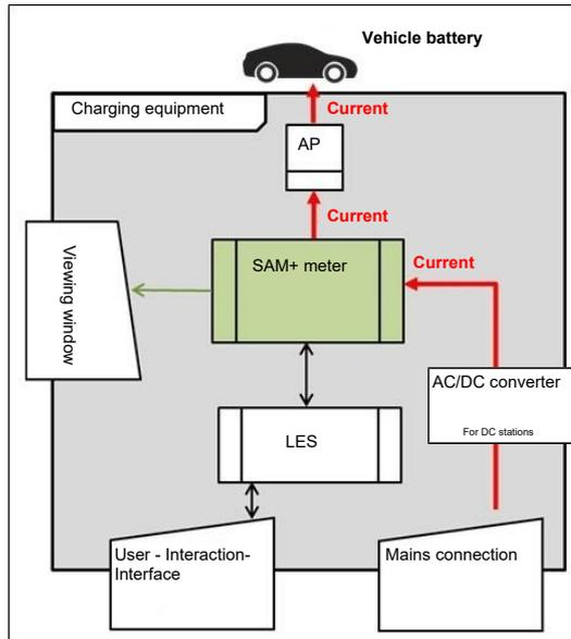
The adjacent image shows the functional arrangement of the SAM (green) in a charging station.
